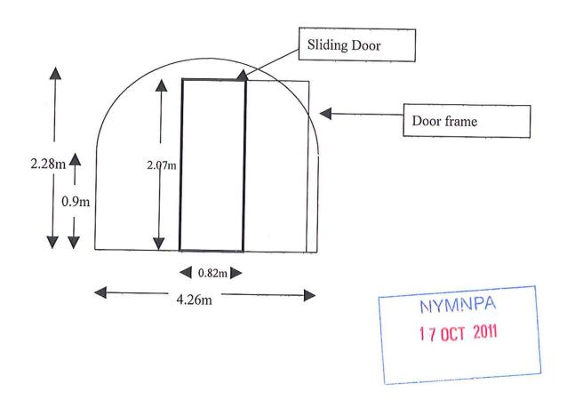
Front and rear elevations with dimensions in metres
