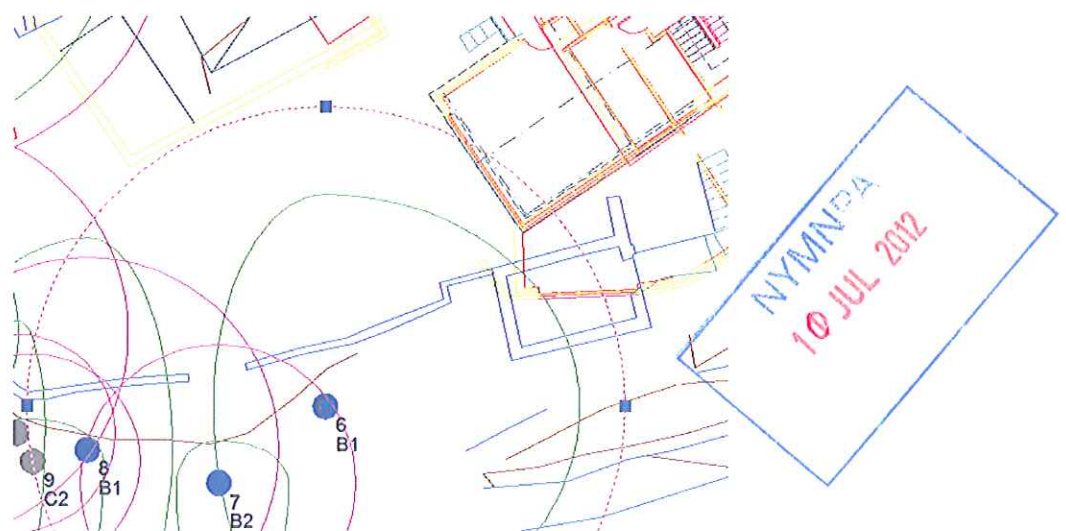
Figure 4: Encroachments within RPA & Proximity of Tree 6 to Approved Structures
