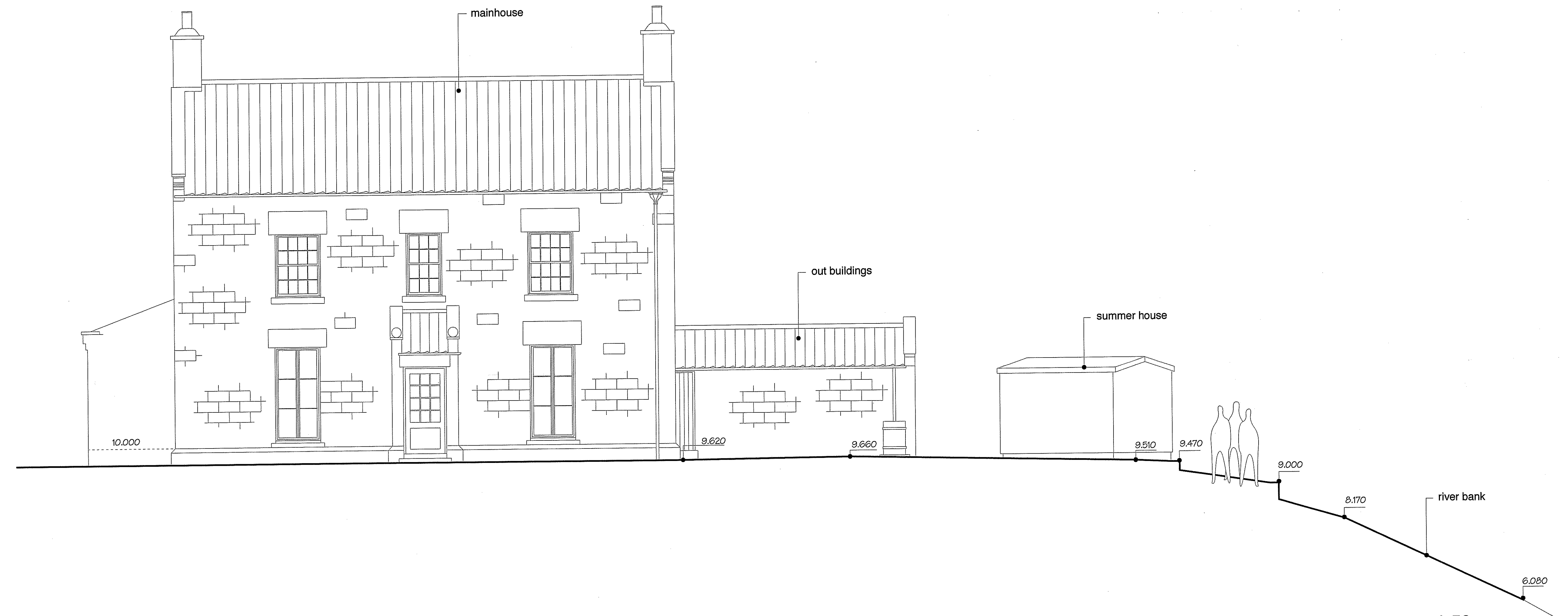
EXISTING ELEVATION TO WEST (hedges omitted for clarity) 1:50
