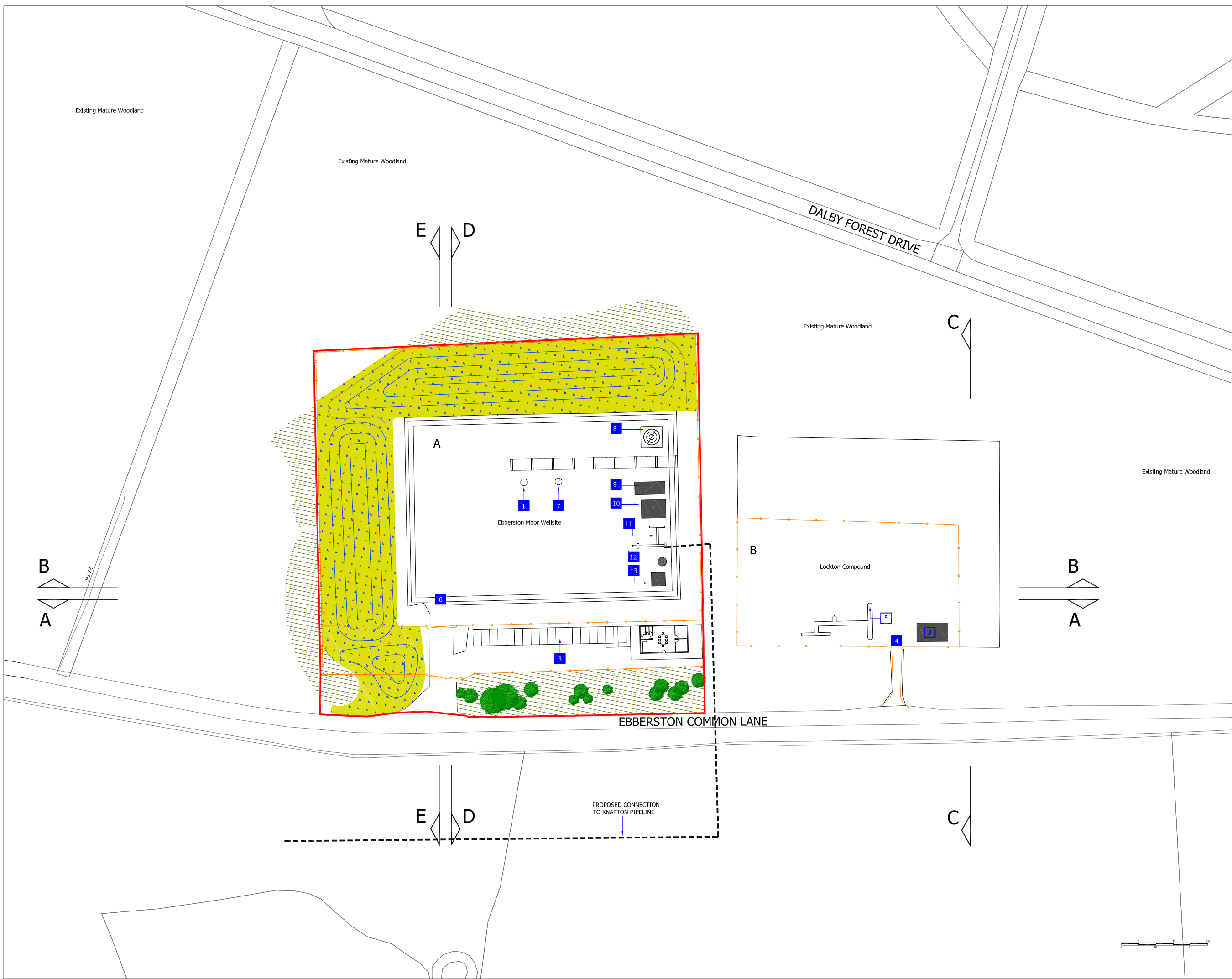
Figure 4.1 DRAFT Project EBBERSTON MOOR WELLSITE TO KNAPTON PIPELINE Drawing Title PROPOSED SITE LAYOUT EBBERSTON MOOR 'A' WELL SITE Date JULY 2013 Scale 1:500@A1 Drawn by YC Check by RP Project No 19819 Drawing No P_05 Revision A
