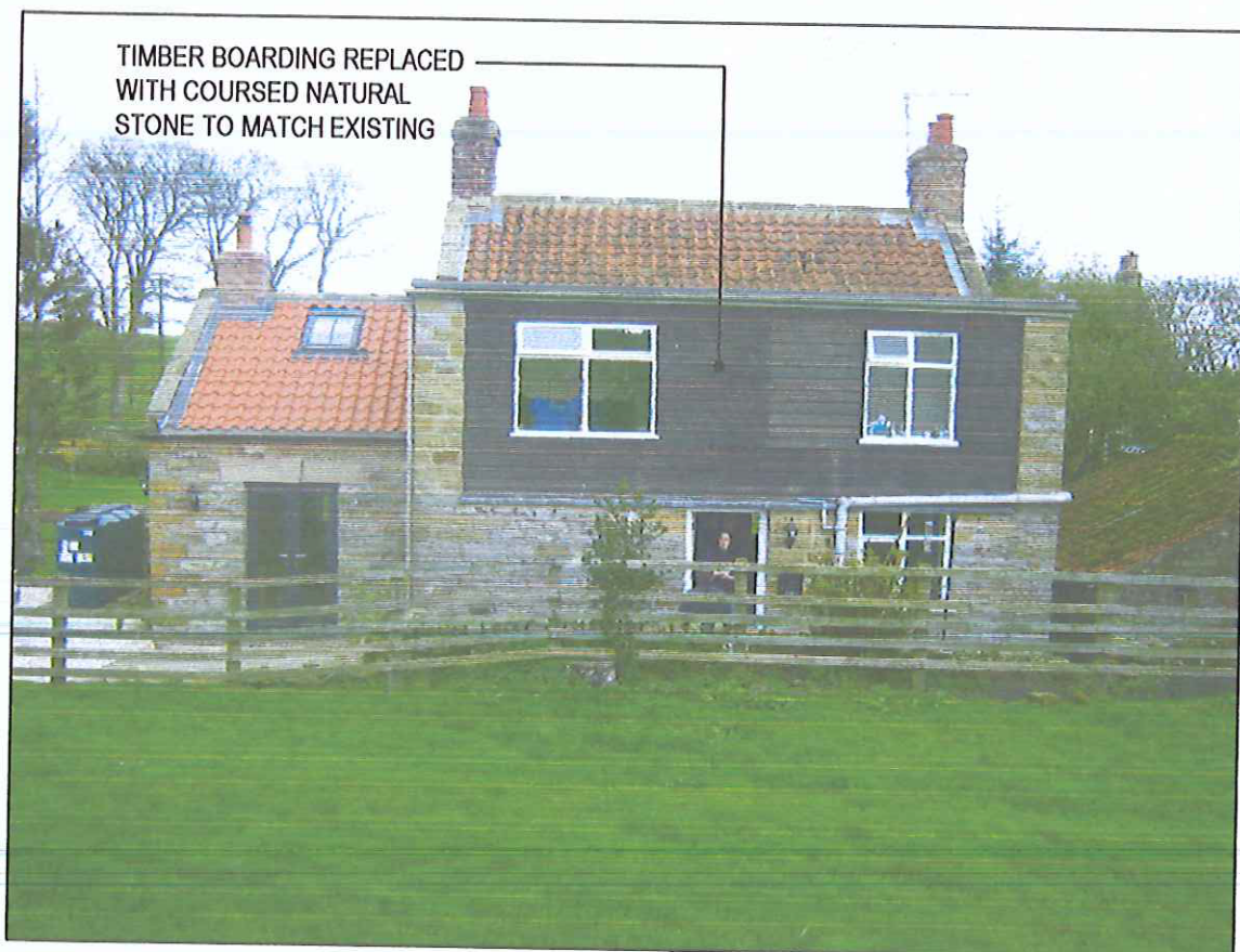
EXISTING REAR ELEVATION
