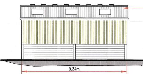
Roof, P6R Fibre Cement Sheeting Colour Natural Grey. 3No. G.R.P. Rooflight Per Side. Vent Ridge Fitted.
