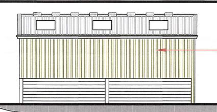
Side Cladding, Vertical Treated Timber Overlapped Boarding From Roof Line To 1.40m Above Floor Level With 1.40m horizontal T&G Stock Walling To Floor.
