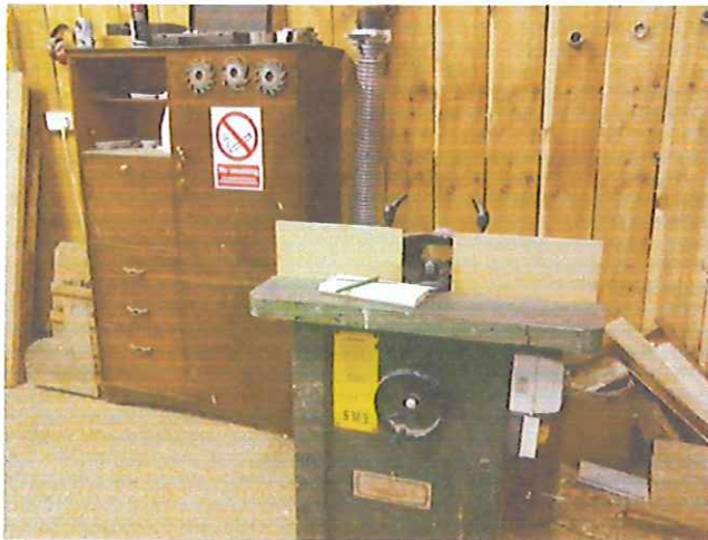
2 nd spindle moulder which I use for rebating, moulding, bevelling, etc.
