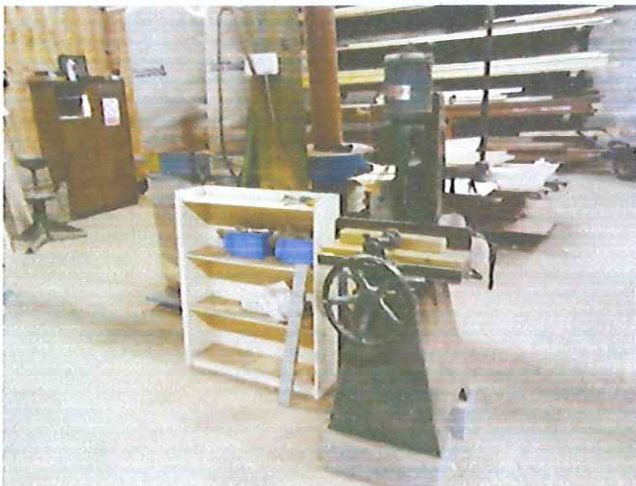
Mortise machine, for making mortise and tenon joints.
