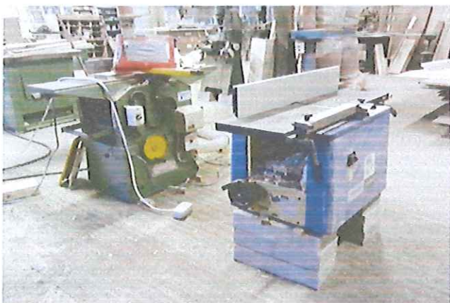
2x planer thicknesser's, used as a pair to save time changing beds, which makes a more sufficient system
