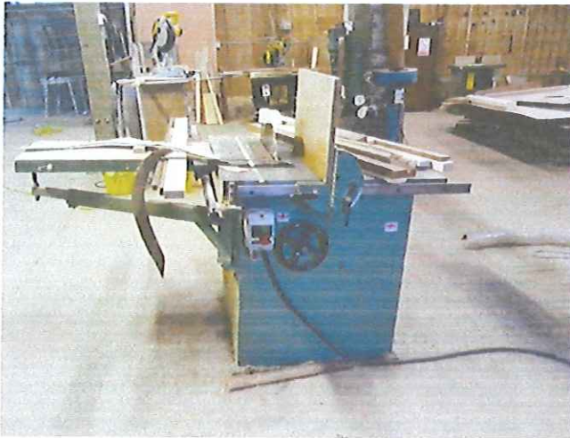
Circular saw, used for ripping lengths of timber.
