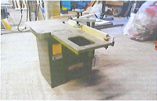
Spindle moulder set for tenoning, so every joint is accurate.
