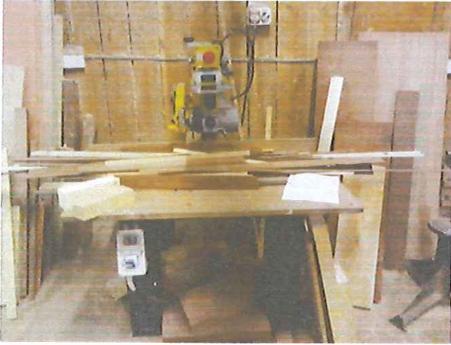
Cross cut saw, used for cutting timber to length and size and cutting shoulders on frames.
