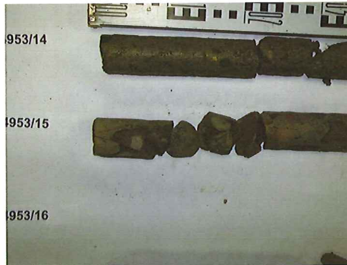
Photo 14 - Detail of core samples 14 - 15 (core 16 missing)
