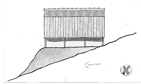
This building is aligned with the contours of the sloping site. Using cut and fill helps to minimise the overall height of the building.
