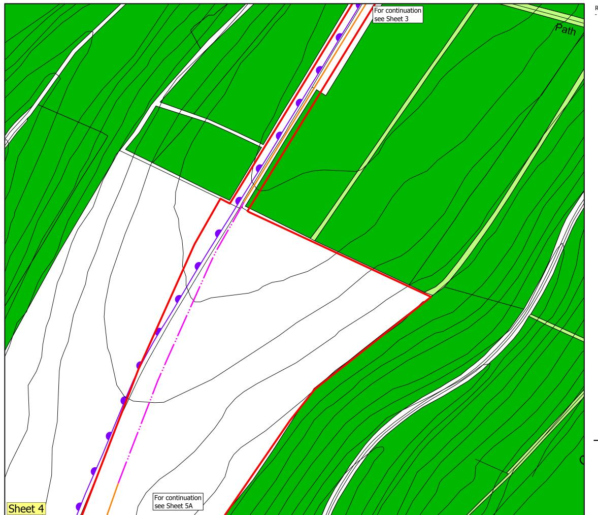
The scaling of this drawing cannot be assured Revision Date Drn Ckd **LEGEND Application Site Boundary** Other Land in Applicant's Ownership North York Moors National Park Boundary Consented Moorland Energy Pipeline Consented Third Energy Pipeline Additional / Modified Sections of Pipeline Key Plan Ebberston Moor South Well Site to **Knapton Gas Pipeline** Drawing Title **Detailed Site Layout** Sheet 4 of 12 Drawn by Check by
