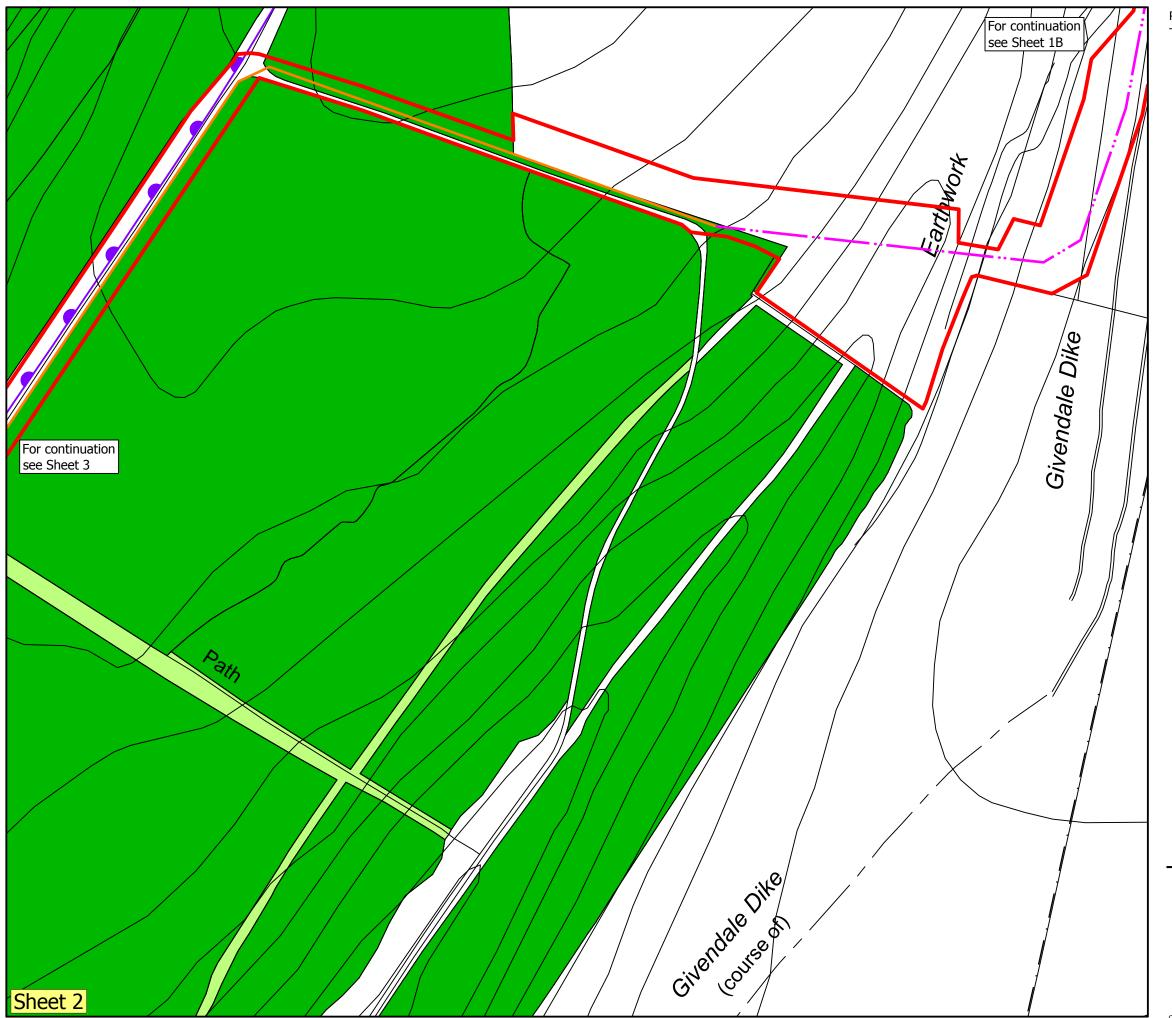
The scaling of this drawing cannot be assured Revision Date Drn Ckd **LEGEND** Application Site Boundary Other Land in Applicant's Ownership North York Moors National Park Boundary Consented Moorland Energy Pipeline Consented Third Energy Pipeline Additional / Modified Sections of Pipeline Key Plan Ebberston Moor South Well Site to **Knapton Gas Pipeline** Drawing Title **Detailed Site Layout** Sheet 2 of 12 Drawn by Check by 05.08.2014 1:2,500 @A3
